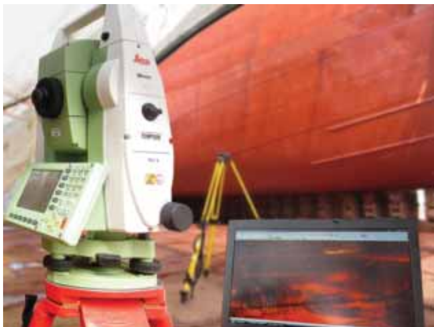
INVESTIGATION WORK: SOMETIMES A 3D LASER SCAN OF THE HULL GEOMETRY CAN BE A NECESSITY TO HELP CHECK HYDROSTATICS AND DRAUGHT MARK POSITIONS.
